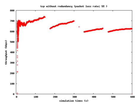
Figure 13 TCP without multi-homing mechanism support
