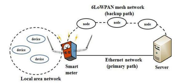
Figure 7 A smart meter network with SCTP multi-homing mechanism
