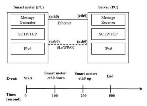
Figure 14 System architecture of the multi-homing experiments
