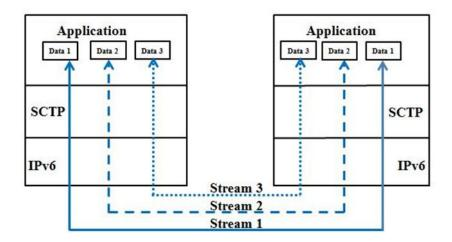
Figure 8 SCTP multi-streaming mechanism
