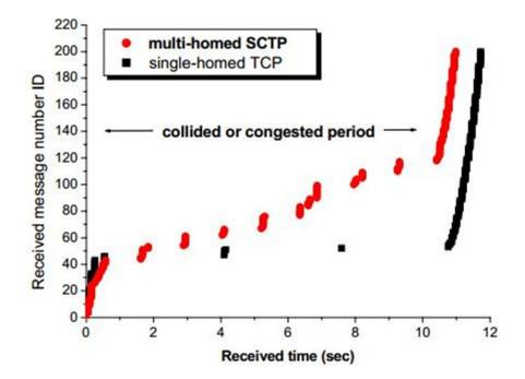
Figure 4 Alternate retransmission of SCTP vs TCP
