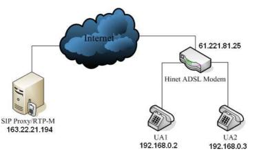
Figure 17: SIP Proxy Server and UAs on different WANs
