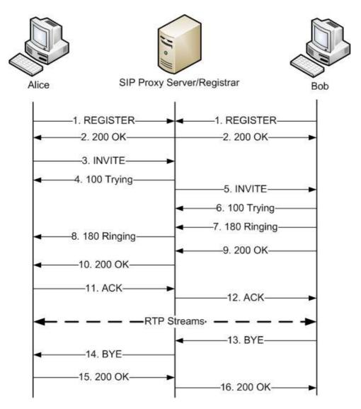
Figure 4: Example of SIP Message Flow
