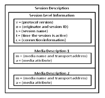
**Figure 6: Structure of SDP**
