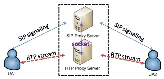
Figure 7: Collaboration of a SIP Proxy Server and an RTP Proxy Server
