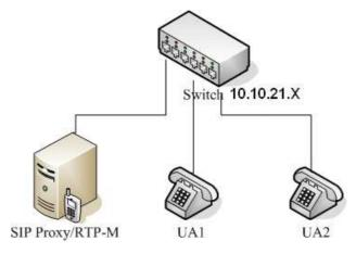
Figure 15: SIP Proxy Server and UAs on the Same Subnet
