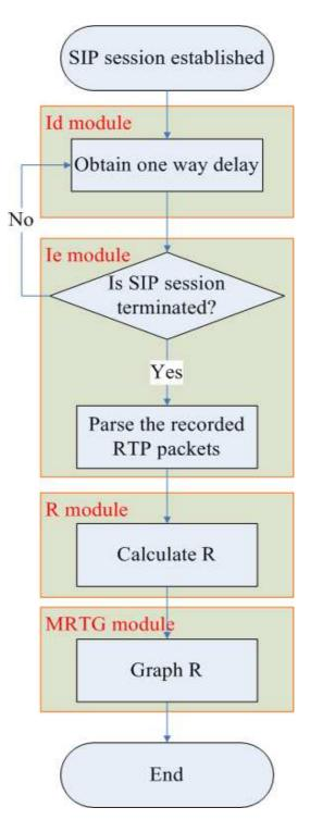
**Figure 9: Flowchart of RTP-M**
