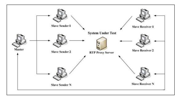
Figure 13: The Architecture of DIST-V [13]
